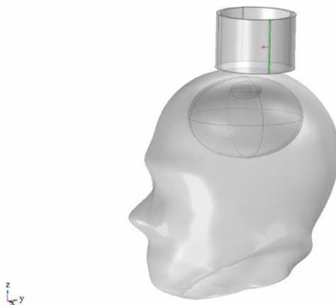
Figure 3. The setting of coil current. The red arrow represents the direction of the input current in the coil. In this direction, the magnetic field generated by the coil is downward to ensure that it can pass through the cerebral hemorrhage area.
