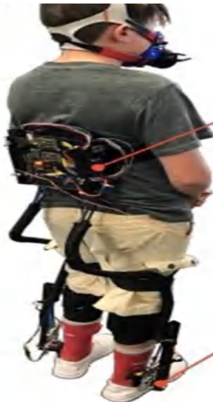
Figure 10. Ankle exoskeleton robot. This figure is cited from [29].
