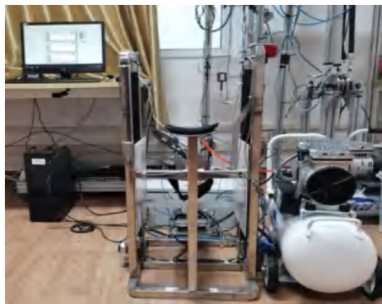
Figure 4. Pneumatic muscle-driven flexible ankle foot rehabilitation robot. This figure is cited from [21].
