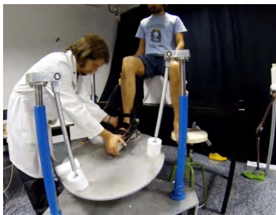
Figure 3. 3-PRS (prismatic-revolute-spherical) parallel robot. This figure is cited from [20].
