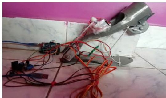
Figure 7. Electric ankle foot orthotics. This figure is cited from [24].
