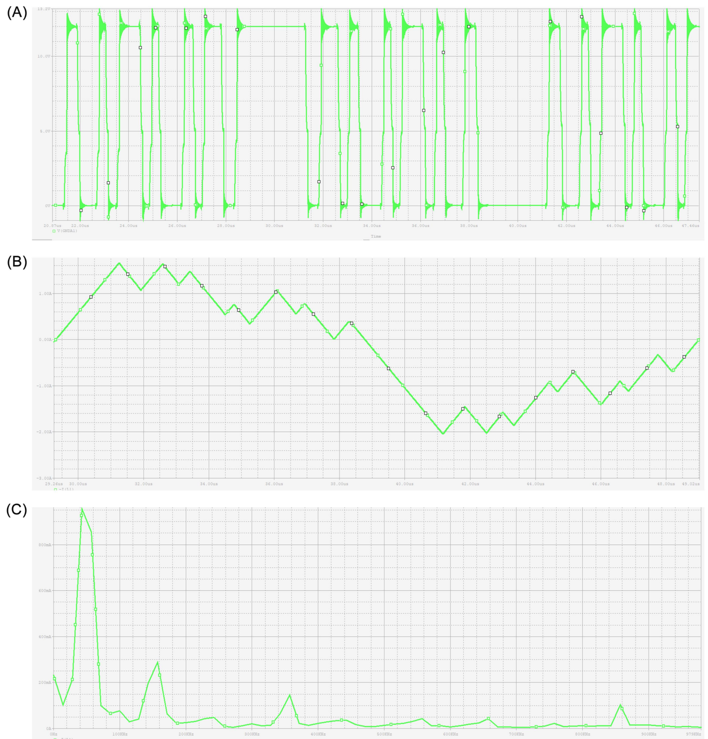
Figure 10. Voltage, current, and current spectrum of the excitation coil from hardware circuit simulation. (A) Time-domain voltage waveform of the H-bridge output; (B) Time-domain current waveform through the excitation coil; (C) Frequency-domain spectrum of the coil current showing multi-frequency excitation peaks at 50 kHz, 150 kHz, 350 kHz, and 850 kHz.
