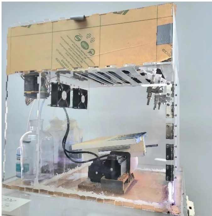
Figure 7. Physical prototype of the staining device.
