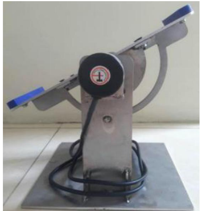
Figure 10. Stepper motor ankle rehabilitation robot. This figure is cited from [25].
