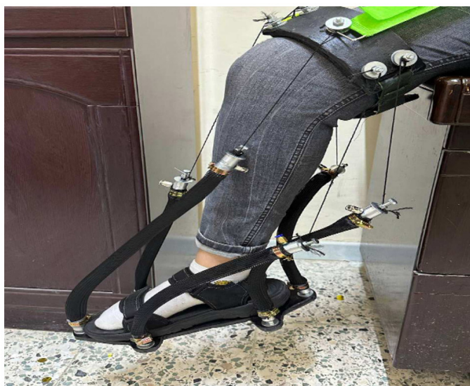
Figure 12. A wearable flexible ankle rehabilitation robot. This figure is cited from [27].
