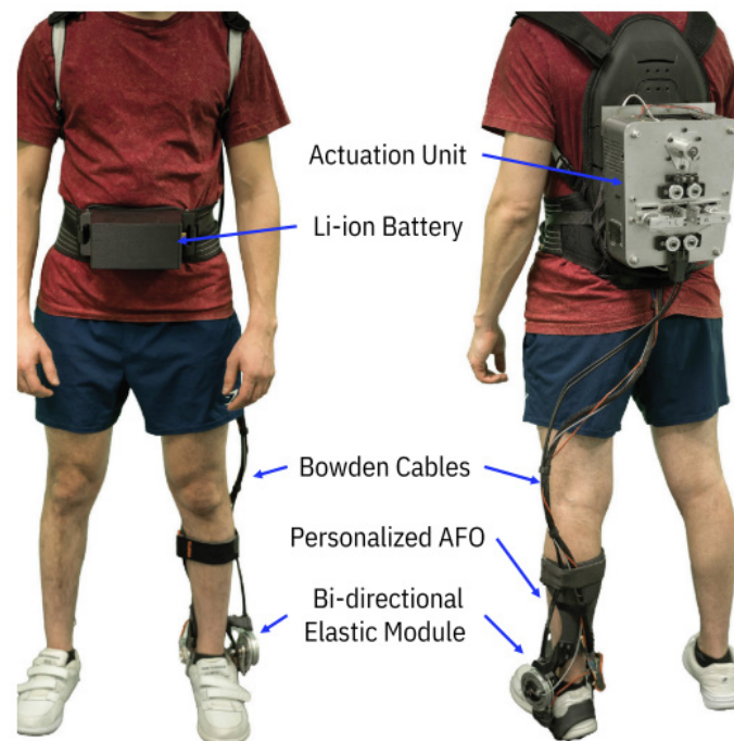
Figure 3. Personalized ankle exoskeleton based on series elastic actuator. This figure is cited from [18]. AFO, Ankle Foot Orthosis.
