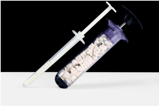
Figure 1. XStat hemostatic injector. The device consists of a syringe (for delivering sponges) and chitosan-coated cellulose sponges (core hemostatic component). The sponges expand rapidly after contact with blood to form a pressure matrix.
