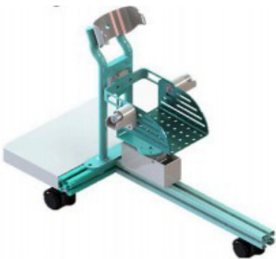
Figure 12. Reconfigurable ankle rehabilitation robot. This figure is cited from [31].
