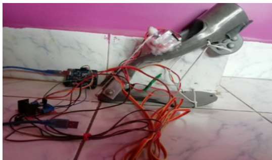
Figure 7. Electric ankle foot orthotics. This figure is cited from [24].
