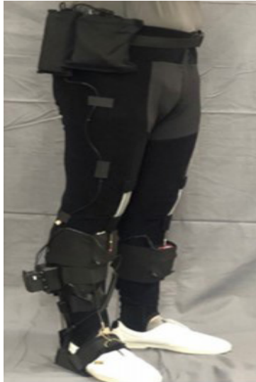
Figure 5. Wearable robot ankle foot orthotics. This figure is cited from [22].
