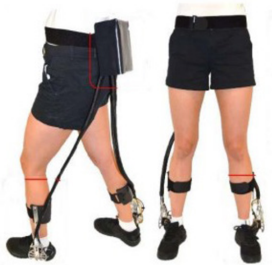
Figure 11. Cable powered ankle exoskeleton robot. This figure is cited from [30].
