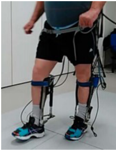
Figure 9. Powered ankle exoskeleton robot. This figure is cited from [26].
