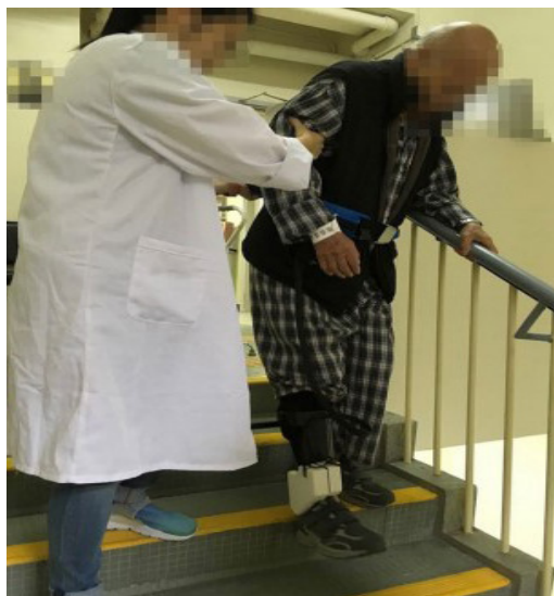
Figure 13. Electric series ankle exoskeleton robot. This figure is cited from [33].
