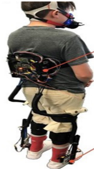
Figure 10. Ankle exoskeleton robot. This figure is cited from [29].
